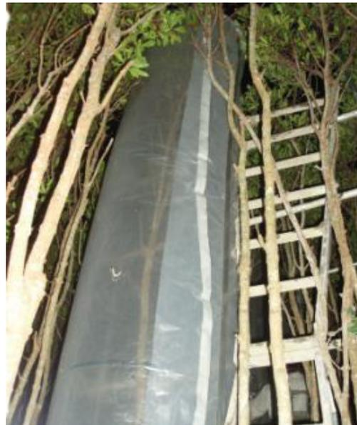
**Photo 3.** Individual aboveground respiration of *Kandelia obovata* trees were measured using a closed chamber method in the field (Hoque et al. 2009, 2010).
